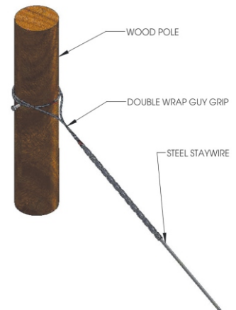
APPLICATION OF DWGG BETWEEN STAYWIRE AND POLE
