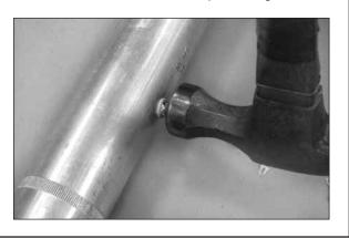
Step #21 Peen over the aluminum edges of the filler hole with a hammer and flat head screwdriver to secure the ball into place.
