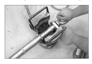
**Step #23** Compress the aluminum body over the steel eye from the "Press First" knurl to the "Stop" knurl.
