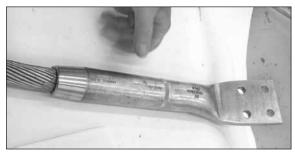
Step #34 Insert the jumper terminal into the press, and compress the conductor starting from the "Press First" knurl moving out to the edge of the tapered end of the tube.
