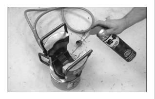
Step #12 Insert the assembly into the compression press. After, ensure the proper alignment of the steel eye with the compression dead-end body.
