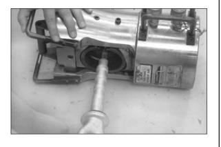
**Step #15** Remove tape from aluminum strands. Check that a gap remains between the aluminum strands and eye.
