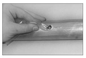
**PLP TIP:** The plastic bag containing the ball should be used to more easily position the ball into place than by hand and to avoid dropping.
