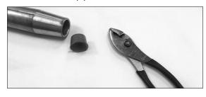
**Step #29** Measure the terminal from the taper to the knurl to check depth.
