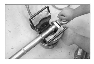
**Step #23** Compress the aluminum body over the steel eye from the "Press First" knurl to the "Stop" knurl.
