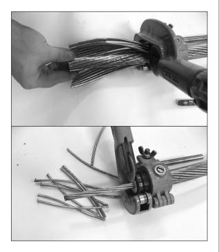
**PLP TIP:** To ensure no damage to the steel core and rapid installation, PLP recommends the use of a Utility Approved Trimming Tool. After strands are removed, any flash or burrs on the outside can be removed with a file.
