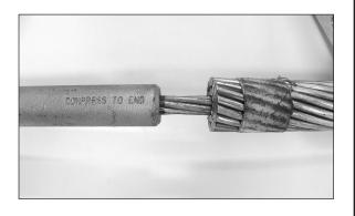
**Step #10** Prepare the compression press and install the die sizes marked on the steel dead-end eye.
