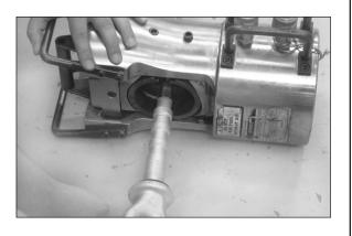
**Step #15** Remove the tape from the aluminum strands. Check that a gap remains between the aluminum strands and the eye.
