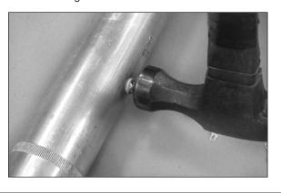
Step #21 Peen over the aluminum edges of the filler hole with a hammer and flat head screwdriver to secure the ball into place.
