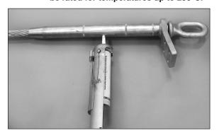
**Step #18** Cease application when the filler compound seeps out the tapered "conductor facing" end of the hardware.
