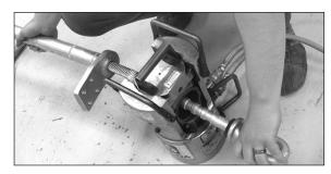
PRECAUTION: TO BE A CORRECT APPLICATION, COMPRESSION CURVATURE MUST BE KEPT TO A MINIMUM, PREFERABLY LESS THAN 1/2 THE ALUMINUM TUBE DIAMETER FROM THE CENTERLINE. FOR THE STEEL, CURVATURE SHOULD NOT BE VISIBLE. EXCESSIVE COMPRESSION HARDWARE CURVATURE IS A MISAPPLICATION OF THE PRODUCT.
