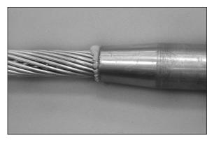
**Step #19** Seal the filler hole by inserting the stainless steel ball.
