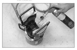
Step #12 Insert the assembly into the compression press. Ensure the proper alignment of the steel eye with the compression deadend body.
