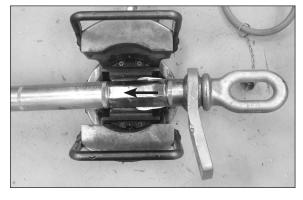
Step #24 After the first section of aluminum body over the steel eye portion is fully compressed, move towards the tapered end/conductor to the second "Press First" knurl.
