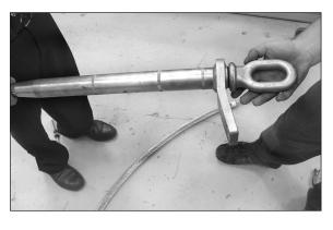
Step #17 Apply appropriate inhibitor (filler) compound through the filler hole in the aluminum body.
