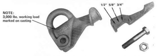
Component Parts. The keeper is to be used with 1/2", 5/8", and 3/4" anchor rods (see arrows). For 1" and 1-1/4" anchor rods, the PREFORMED<sup>TM</sup> Pulling Eye is used without the keeper.
