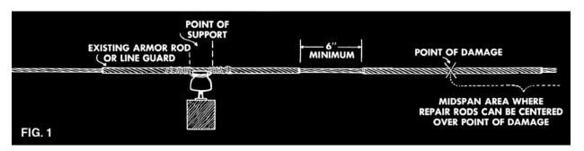
When centered over the point of damage, the ends of the *Conductor Splice* should not be positioned closer than 6 inches to existing *Armor Rods* or *Line Guards*. The Restorative-Repair function of this splice should be limited to damage located within the "Midspan Area" or the "Point of Support". (See Figure 1)
