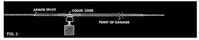
The *Armor Splice* combines the features of both *Armor Rods* and *Conductor Splices*, which are described in their respective catalog sections. The *Armor Splice* should be considered when damage occurs in the "support area," or where installation would locate the ends of repair rods within 6 inches of existing rods.
