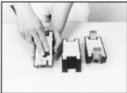
FIGURE 12 - SCUFFING CABLE OPENINGS
