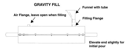
For gravity filling attach funnel with tubing to filling flange. Install plugs in Air Flange and Filling Flange after filling closure.
