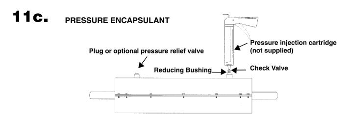
If desired, pressurize encapsulant immediately after gravity filling.
