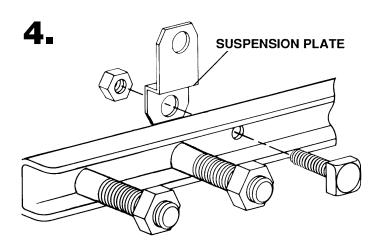
Aerial applications require that the suspension plates be installed to the back LOCKBAR™ Fastener prior to its application to the Shell. A special third hole is provided on either side of the back LOCKBAR Fastener assembly for this purpose.
