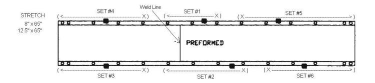
Using an in-lb torque wrench, tighten the nuts according to the sequence shown.
