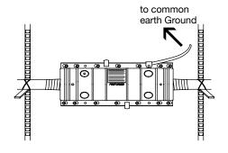
ARMADILLO Stainless should be installed between the manhole racks.
