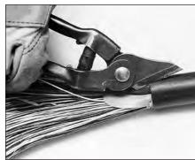
The Pair Protector is a plastic shim that is inserted between the cable shield and the core wrap prior to bonding or tabbing. It allows easy insertion of the bottom shoe of most common shield connectors, and eliminates the danger of cut pairs while cutting tabs in the cable sheath.
