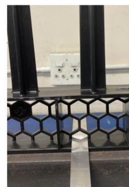
Stainless steel straps are fastened through the honeycomb base design and around the angle iron.
