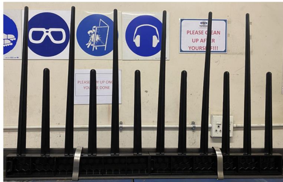
Stainless steel straps are fastened over the BG, through the verticals, and around the angle iron.
