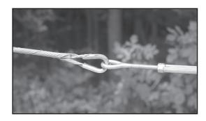
Step #2 If PLP's Heavy-Duty Thimble with the captured tab is being used, bend the tab with pliers or similar hand tool.
