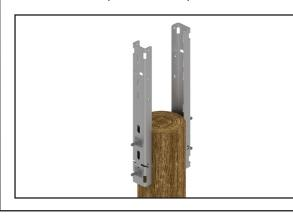
Step #2 (OPTIONAL) If using the optional nest retention posts, attach each nest retention post to the platform frame using a nylon lock pin. Push the pin all the way through the pre-drilled hole from the outside of the frame toward the inside.
