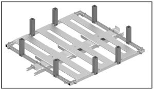
Step #3 (OPTIONAL) If using the optional perch, attach the perch to the tab of the main support bar of the platform. Secure the perch to the tab with a carriage bolt, flat washer, lock washer, and hex nut as shown in Figure 1. Secure the perch to the main support bar of the platform with a hex head bolt, lock washer, (2) flat washers, and a hex nut as shown in Figure 2.
