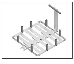
**Step #4** Secure the platform to each pole top bracket with (2) carriage bolts, (2) flat washers, (2) lock washers, and (2) hex nuts as shown below. Go back and fully tighten the 5/8" through bolts.
