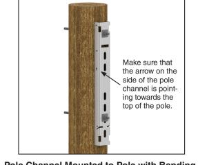
Pole Channel Mounted to Pole with Banding
