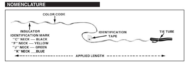
**Tie Tube:** Each tie is furnished with Tie Tube Component. The Tie Tube is detached and applied over the conductor.
