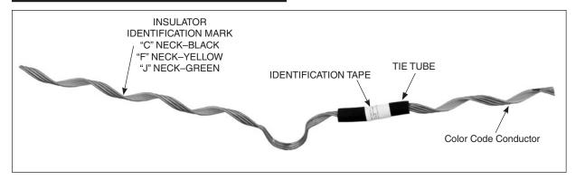
**Tie Assembly**: An Alloy Spool Tie Assembly consists of one metal tie component plus tie tube.
