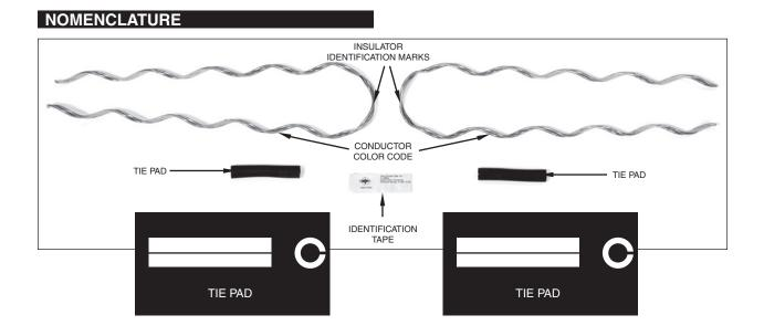
**Tie Assembly**: An Alloy Double Side Tie assembly consists of two aluminum tie components plus two tie tubes.
