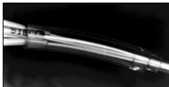
FIGURE 7 - INSERT PIGTAILS INTO PIGTAIL TUBE ASSEMBLY
