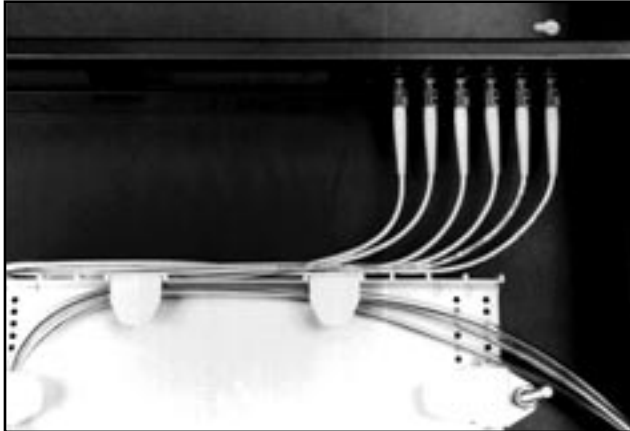
FIGURE 5 - ROUTE THE PIGTAILS
