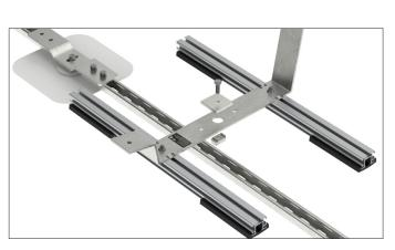
Start by laying the Unistrut next to the roof anchor. With the Unistrut sections in place, lay the Seismic Attachment Bracket over the roof anchor stud. If necessary, use 1 or 2 square washers to shim the Attachment Bracket. Next, slide the Unistrut channel nuts into the Unistrut rail, aligning the channel nut holes with the Attachment Bracket holes. Tighten the flange nut and hex bolts. Torque to 20 ft-lb.
