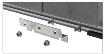
Attach the Inverter Mounting Bracket to the ballast supports using the provided T-bolts and Flange Nuts. Torque to 15 ft-lb.
