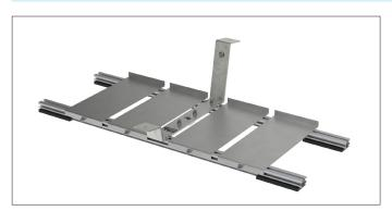
Attach the optional ballast trays to the ballast supports using the provided T-bolts and Flange Nuts. Torque to 15 ft-lbs.
