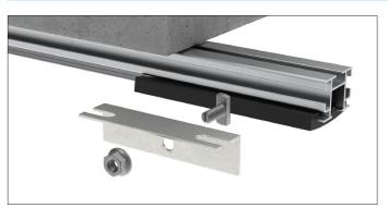
The POWER MAX™ Plus system is capable of supporting conduit runs by installing optional conduit brackets. Install the brackets into the ballast supports by using the provided T-bolt and flange nut. Torque to 15 ft-lb.
