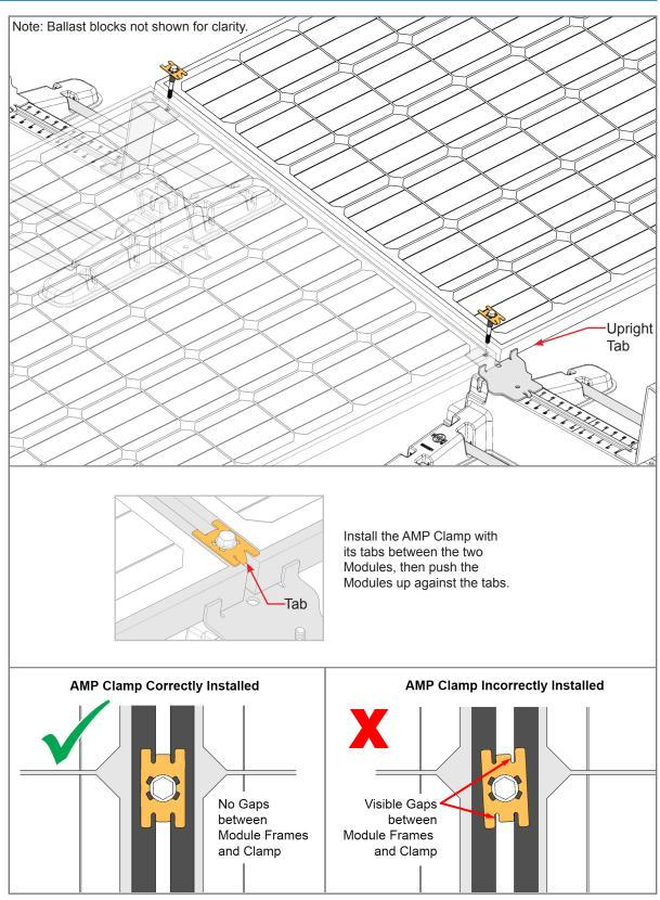
Install one AMP Clamp bonding Mid Clamp assembly into each Bracket. Ensure that the Clamp is square to the Module frames and there are no visible gaps. Tighten the Bolt and **Torque to 15 ft.-lbs.** Continue in the manner installing the remaining Modules.
