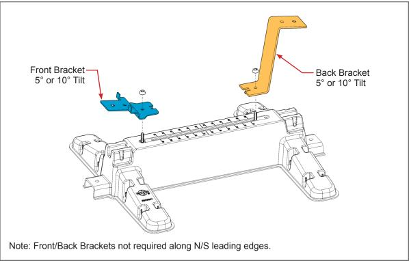
Install the Brackets as shown above. Secure with 5/16-18 Flange Nuts. Torque to 15 ft.-lbs.
