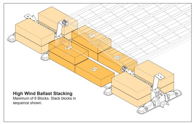
Stacking method for "High Wind" ballast shown above. This does not apply to all systems; only those installed in areas where higher winds require additional ballast.
