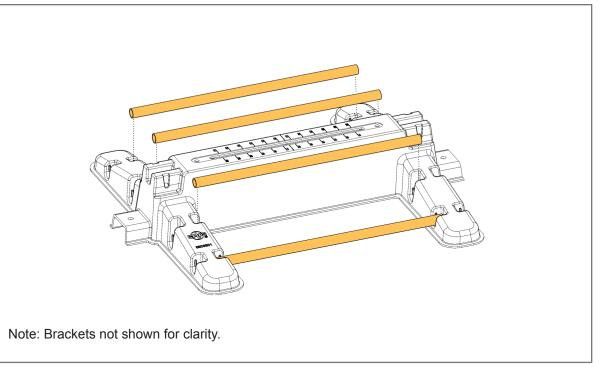
Install each of the four Ballast Support Tubes in their respective notches of the Tray.
