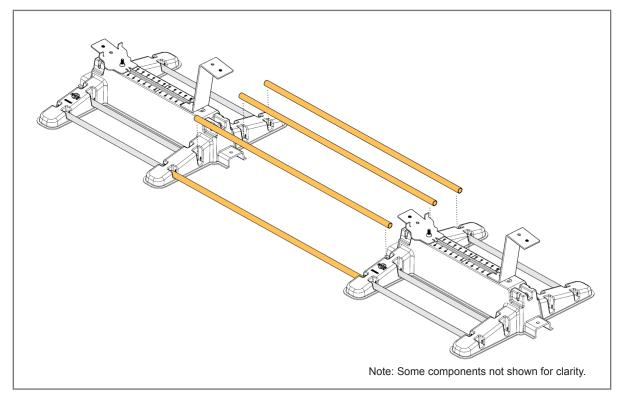
Install each of the four High Wind Ballast Support Tubes into their respective notches of the Tray.
