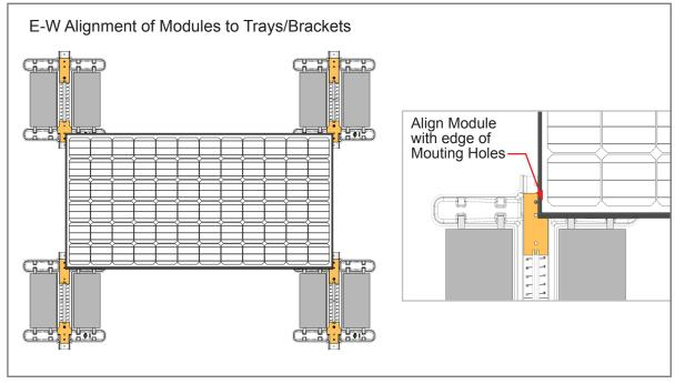
The Trays and Modules relative east/west positioning is established via the mounting holes of the Front and Back Brackets. Align the Module Frame as close as possible to the edge of the threaded mounting holes while leaving just enough clearance to thread the Bolt/Sleeve of the Module Clamps into the Brackets.
