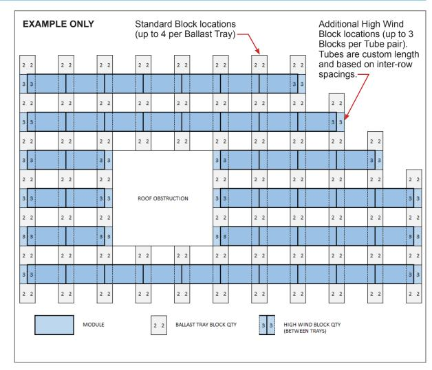
This sample layout shows the specific number of Ballast Block required per Tray by Tray location. These numbers will range from 1-4 blocks. For further details on minimum/maximum block quantities and arranging of ballast blocks, refer to project specific drawing.
