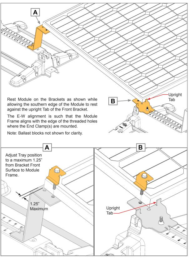
Install one End Clamp assembly into each Bracket. Ensure that the Module is square to the Trays and there are no visible gaps between Sleeve of End
