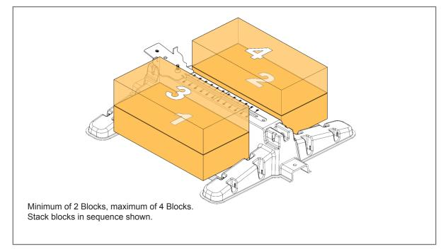
Install the required Ballast per the job specific ballast requirements.
