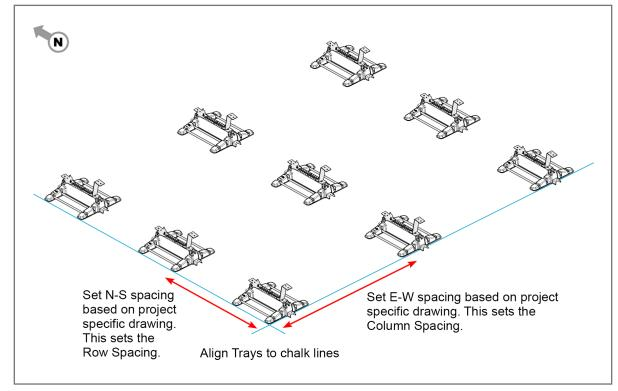
Position the southernmost and (in this example) the westernmost Trays along their respective chalk lines, roughly spacing the Trays as shown. Roughly place
