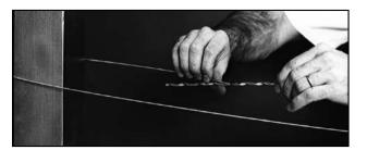
Step #2 After the wire is wrapped around a stake or pulled through a dead-end, start applying the Connector to the tail end of the wire. Be sure to start the application at the center mark on the Connector.
