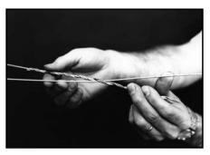
Step #3 Pull the Connector and wire until the wire is tight, and wrap the other half of the Connector onto the wire.
