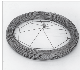
3. Twist at least 2" of the legs together until the wire cage is tight.
