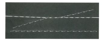
Position the second subset so that the center marks match. Wrap on one pitch length on each side of the center mark.
