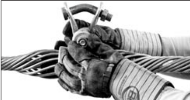
FIGURE 8 - SLIDE BOLT INTO POSITION, APPLY LOCK WASHER
