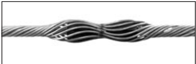
FIGURE 6 - TWIST ALL ROD ENDS INTO POSITION SIMULTANEOUSLY
