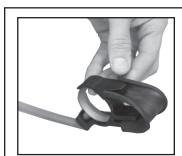
Step #6 Secure the free end of the tube under the short single finger to complete the preparation of the installation tool.
