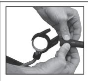
Step #2 Open the tube at one end flattening it in preparation for insertion in the double finger side of the Tube Applicator.
