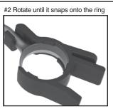
PRELIMINARY Install Tie Tube Applicator to Applicator Ring Tool
