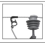
Step #2 With the tube partially on the conductor and still between the double fingers, slide it towards the insulator.
