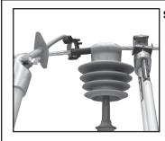
Step #5 Make sure the tube is in the correct orientation with the tube between the conductor and the insulator. Use an edge on the tool to push the tube into place.
