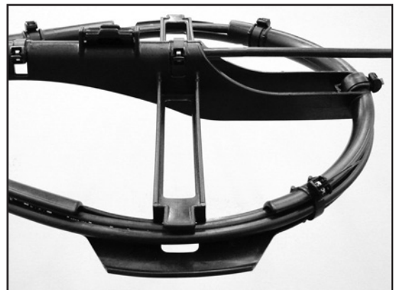
FIGURE 19A: CABLE LOOPS SECURED ON SAME PLANE
