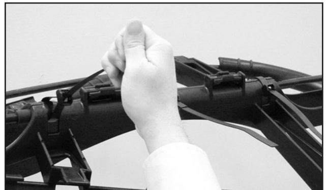
FIGURE 16: SECURE CLAS WITH CABLE STRAPS
