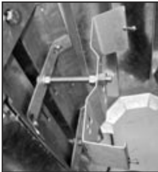
FIGURE 23 - LIMIT EXPOSED THREAD LENGTH
