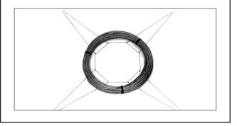
Step #4 Insert a tool (preferable a long-handled screwdriver) through each of the four legs and twist the legs into a "knot". It is not necessary to tighten down the legs all the way. As long as the legs are firmly knotted the dispenser is secure.
