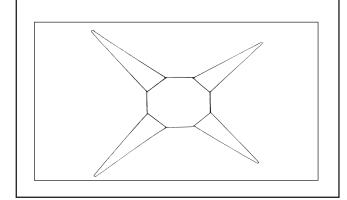
Step #3 Fold the legs of the dispenser over the coil. Legs overlap each other by 2" so that they can be twisted together to secure the dispenser. If legs are not long enough by themselves, tie wire can be used to secure.
