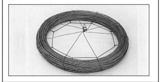
Step #7 After sufficient strand has been drawn out and cut, the loose end should be placed back in the dispenser. The loose end is now secure and the coil can be moved safely.
