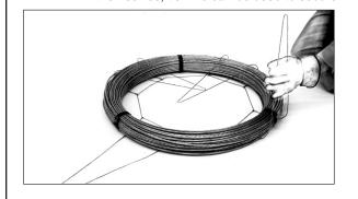
Step #2 With all four legs of the dispenser unfolded lay it on level ground. Place the banded coil of strand on top of the dispenser. Be sure the coil is centered on the dispenser.
