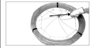
Step #5 The banding on the coil should be cut so that the coil can loosen and expand to fill out the cage of the dispenser.
