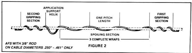
Install the second gripping section by wrapping it around the cable and snap the end of the gripping section in place.
