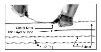
**2.00** Tape the ends of strand with a thin layer of tape. Use the subset of the PREFORMED Splice which contains the greater number of rods and begin the application as shown.
