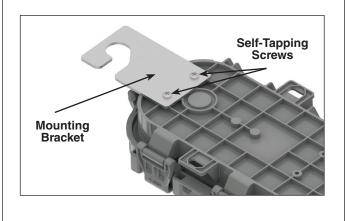
**Step 2:** Hang the closure from the offset ladder bar of the pedestal bracket with the mounting bracket, as shown below
