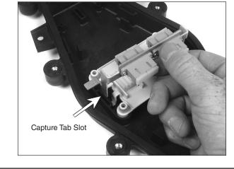
Step #43 Install connectors into adapters.
