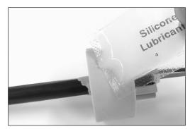
Step #13 Insert grommet into closure base and insert strength member of cable through the slot of the "L" bracket.
