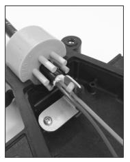
Step #14 Crimp "L" bracket with side cutters to secure strength member.
