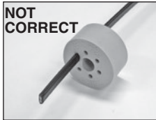
Not Correct Installation
