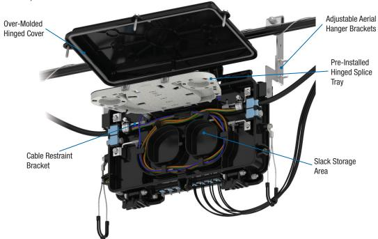
The COYOTE<sup>®</sup> ATC has a pre-installed 48 CT. single fusion hinged splice tray that allows access to underlaying slack storage. The splice blocks can accept single fusion or mass fusion splices as well as pre-connectorized splitters. A pass-through window allows either pigtails or splitter outputs to pass to the drop chamber. Once the splicing has been completed the splice chamber cover is secured using three pre-installed bolts to restrict access.
