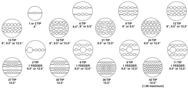
\*NOTE: These are custom-drilled End Plates. Only the most common combinations are shown. Since the End Plates are custom-drilled, almost any combination is possible. Contact PLP for a TIP CABLE Mea-SURE™ Tape P/N 02922 at the sales office at: 440-461-5200.
