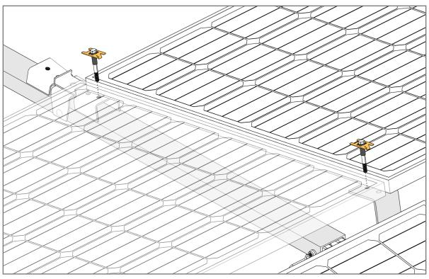
Install one AMP Clamp bonding Mid Clamp assembly into each Bracket. Ensure that the Clamp is square to the Module frames and there are no visible gaps (see previous page). Tighten the Bolt and **Torque to 15 ft.-lbs.**
