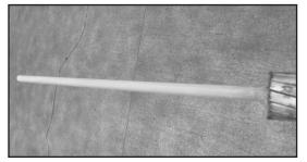
**PLP TIP:** To prevent damage to the composite core and speed installation, PLP recommends using a conductor trimming tool.
