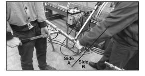
Step #13 Bring the two sides together and handtighten the swivel end of the coupling to the collet retainer. Use a torque wrench to fully tighten to a minimum of 85 ft-lb (115 Nm).
