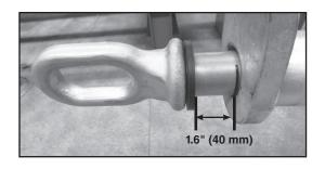
Step #14 Position the inner aluminum sleeve so that 1" (25 mm) of the filler tube is sticking out or it is stopped by the indent.
