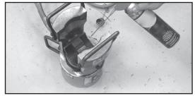
Step #16 Begin compressing on the outer aluminum tube at the opposite end of the eye, making sure that the correct die size is being used. Slightly overlap crimps in the direction of the eye to ensure complete compression. Continue to compress until the compressions meet the stop mark on the outer aluminum tube.
