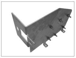
Step #2 Before attaching the Defender Vertical Bracket Component (from SP2906) to the structure, attach the Dome VMB to the holes at the bottom using the 5/8" bolts, lock washers, and nuts.
