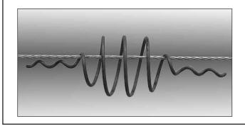
**Step #4** Wrap the gripping section on both ends around the conductor or strand.
