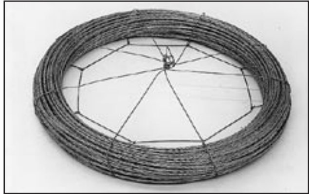
Figure 7 - Cut banding on the coil so it can expand and fill out the cage of dispenser
