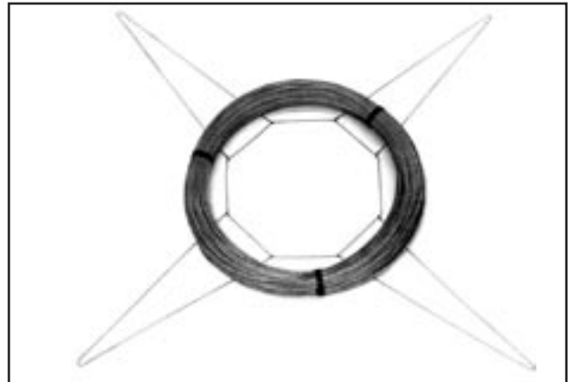
Figure 3 - Place banded coil of strand on top of the dispenser
