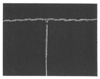
Shown: A completed application of the PREFORMED Reducing T -Connector.
