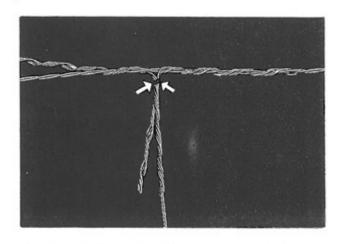
4. When applying the Reducing T -Connector be sure to apply the marked leg to the smaller diameter strand. The marks on the Reducing T -Connector will phase in with each other at the end of the vertical strand as indicated by the arrows. Position the second element on the strand so that the upper leg passes under the horizontal strand and the lower leg passes over the vertical strand as shown. Wrap on both legs completely.
