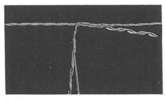
3. If the strands are of different diameters the Reducing T -Connector must be used, and the marked leg must be applied to the smaller diameter strand. Position the first element on the strand so that the upper leg passes over the horizontal strand and the lower strand leg passes under the vertical strand. Be sure that the vertical strand does not come in contact with the horizontal strand. Wrap on each leg one or two turns as shown. Then wrap on the legs completely.
