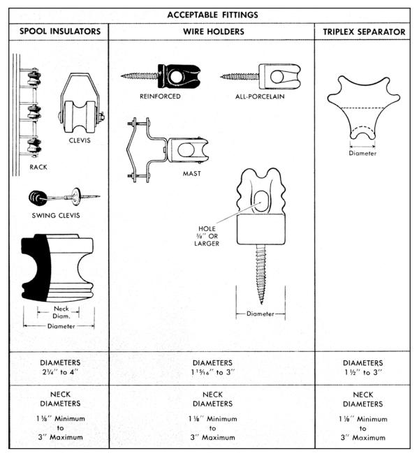
Loops of the **Service-Grip Dead-end** are designed for use with a variety of porcelain fittings. These fittings are recommended because they have smoothly contoured diameters between 1-1/8" minimum and 3" maximum. Refer to catalog pages for maximum neck diameters for specific Service-Grip Dead-ends.
