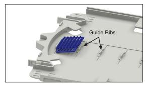
**Step #2** Insert the microtubes into the slot(s) of the LITE-GRIP Sleeve.
