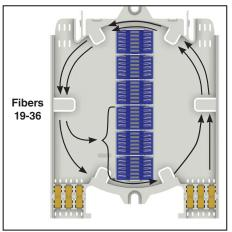
Step #3 Insert the LITE-GRIP Sleeves into the entry channel and confirm that each sleeve is inserted between the guide ribs.
