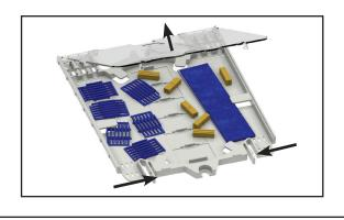
Step #4 Insert the plastic splice blocks between the guide ribs and confirm that the tabs of each splice block are captured within the slots of the guide ribs.
