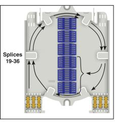
Step #6 Install the cover onto the tray by first capturing the legs of the cover under the tabs of the tray. Once the legs are captured, rotate the cover downward until the locking tabs of the cover snap into place in the tray.
