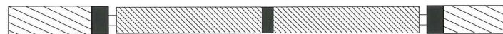
B) Filler Rods: Sub-set or single rods, not gritted. The filler rods may not be required for certain sizes of conductor
