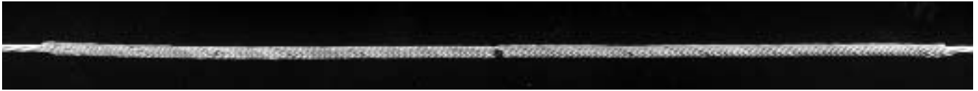
7) Splice completely applied
