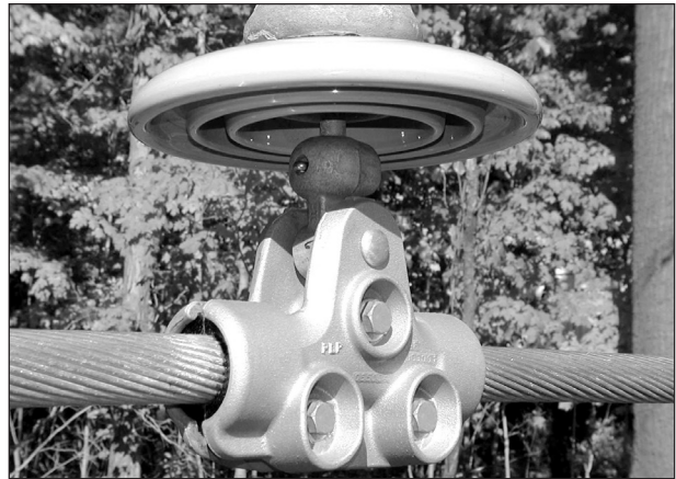
Completed application of the CUSHION-GRIP® Suspension. The work hole located on the bottom of the clamp has a maximum working load of 500 lbs.
