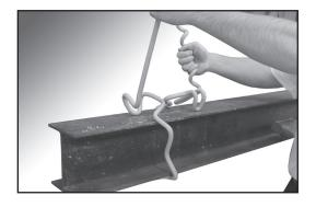
**Step #3** Lifting on the uprights, flex them away from each other to snap the hooks over the top edges of the I-Beam.
