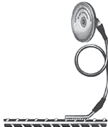
Earthing Bond on Ribar
