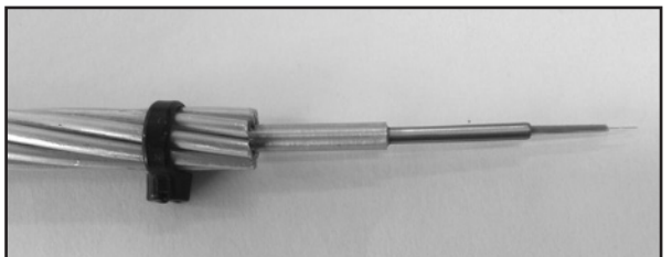
Type 4: OPGW with Central Aluminum Tube with or without Central Stainless Steel (Ridged) Buffer Tube – This is similar to Type 3 but optical fibers are housed in a central aluminum tube or a single stainless steel buffer tube within a central aluminum tube
